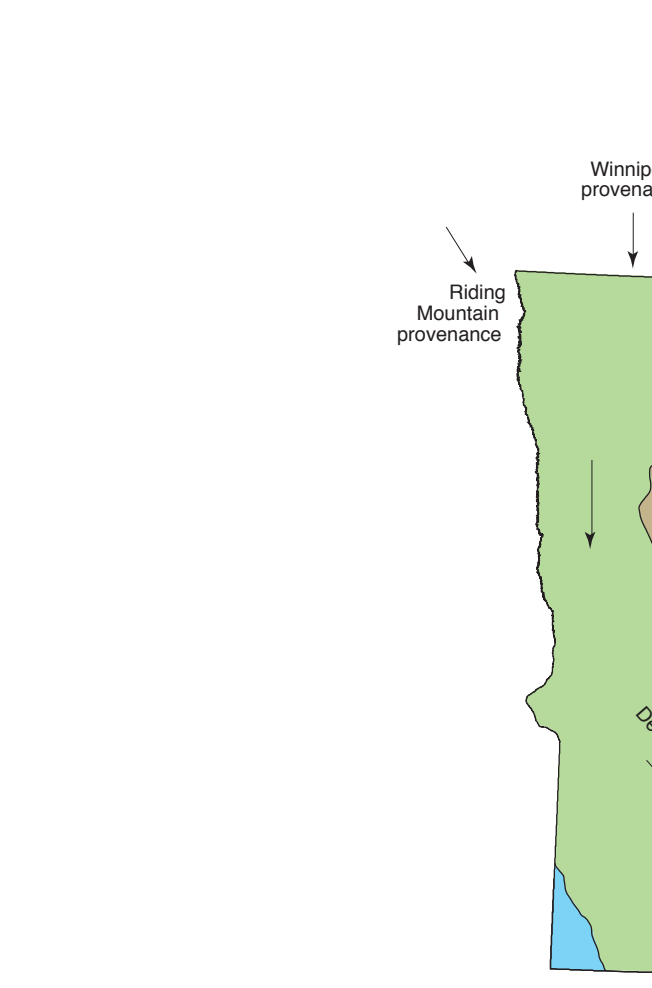
Figure 2. General flow paths of glacial ice from the four provenances towards Dodge County. The flow paths for the Winnipeg and Rainy lobes are nearly identical south of central Minnesota. The flow path for the Des Moines lobe is very similar to the Winnipeg and Rainy lobes. Because the ice incorporated additional rocks while flowing along these similar flow paths, the glacial deposits in southeastern Minnesota tend to have more mixed and therefore less diagnostic lithologic compositions than deposits in central or northern Minnesota. Modified from Meyer (2000).
