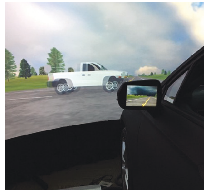
A moving pickup truck crosses the participant vehicle in a sight estimation test at the U of M lab.
