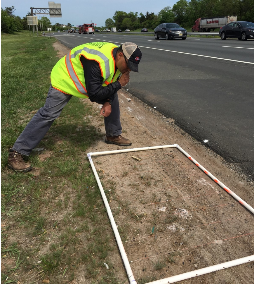
Figure 3.1 Grid overlaid on a plot in New Jersey. Each grid intersection was logged as being on top of the turfgrass that was originally seeded, a weed, or bare soil.
