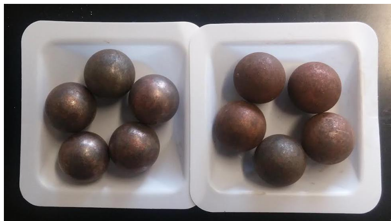
Figure 1.46. The condition of used Chrome-Iron balls after one use (left) and after two uses (right).
