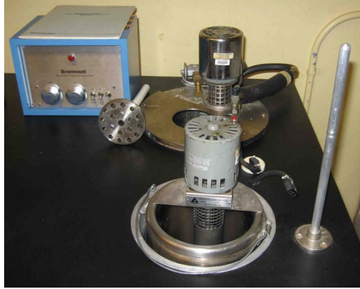
Figure 4.13: Rosemount Temperature Calibration Facility
