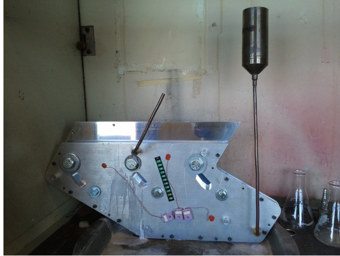
Figure 4.22: Assembled Mass Transfer Plate During the Casting Process
