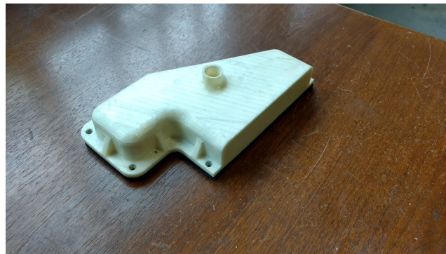
Figure 3.12: Discrete Hole Plenum
