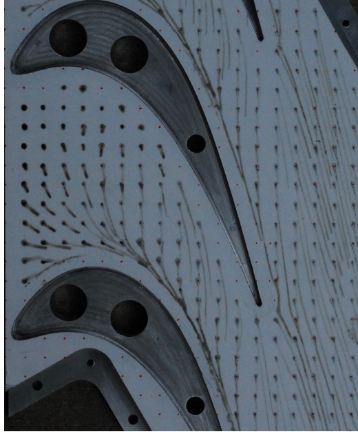
Figure 5.14: Endwall Flow Visualization
