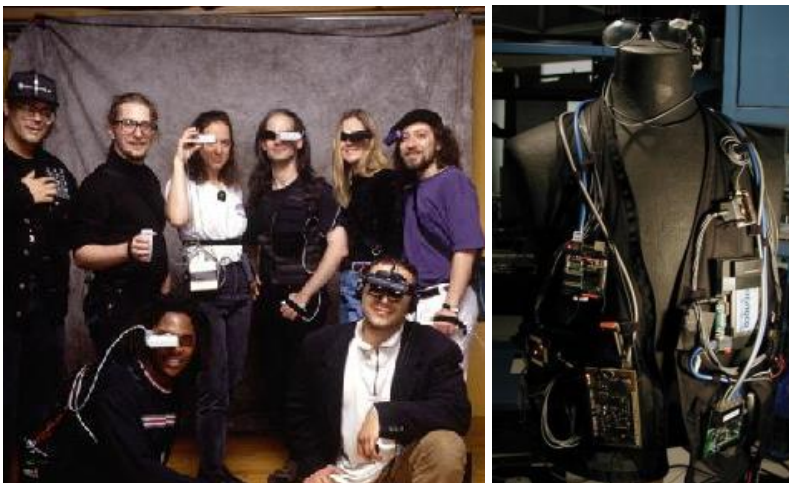
Figure 3.- 4. (Left) MIT's wearable computers in the 1990s and (Right) MITHril Vest in 2003 ("Wearable Computing at the MIT Media Lab," n.d.)
