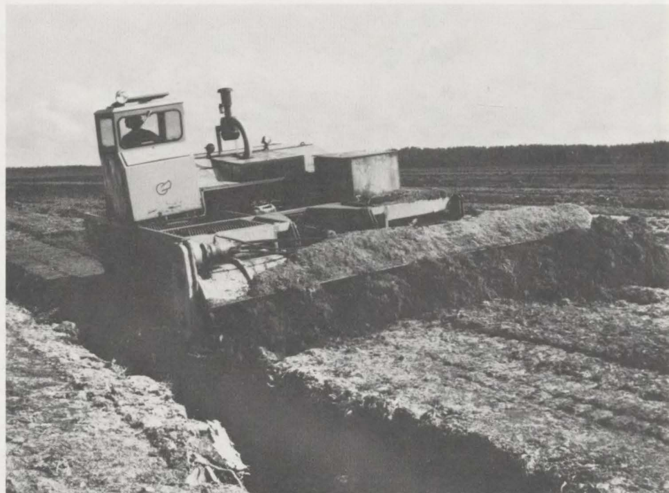
Ditching (left), the first step in the mining process, is necessary to drain the peatland so it can support heavy equipment such as the leveling machine (right), which prepares the surface of the peatland for mining.
