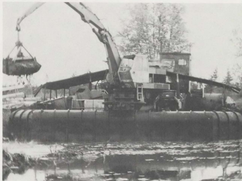
Hydraulic peat mining in British Columbia, using a clamshell dredge on a hovercraft barge.
