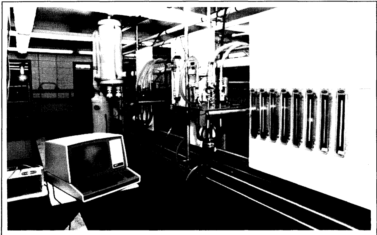
Figure 1. The "mechanical cow" data acquisition system is shown in the lower left corner. Water flow rotometers for unit 1 are shown at the extreme right, and unit 1 with individual water flow control is adjacent to the rotometers. Unit 2 is further back and adjacent to the closed circuit water circulation system simulating internal udder pressure (2 vertical tanks). Note the stainless steel milk pipelines, one below the milking units, the other above the fluorescent lights.
