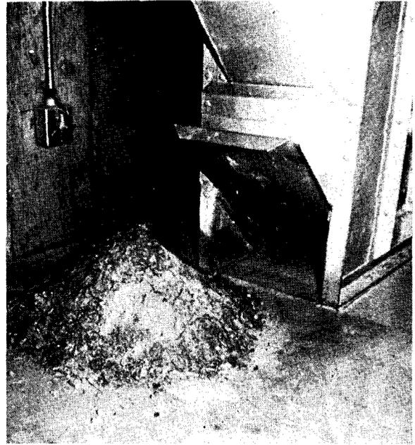
**Figure 3.** Elevator legs can hold sizable amounts of residual feeds or ingredients. Some of this material can be incorporated in the next batch of feed.
