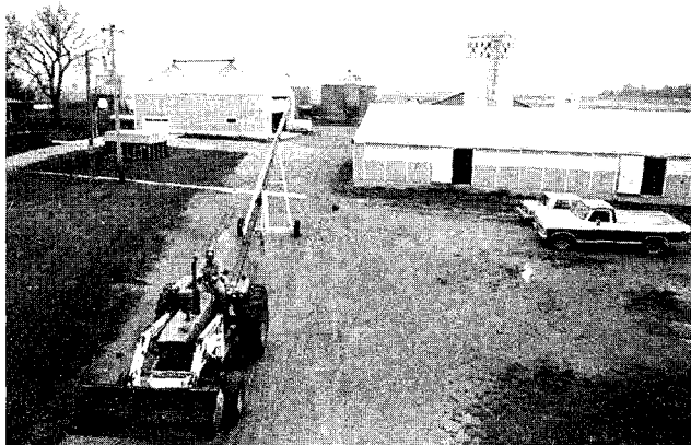
Make sure tall pieces of equipment can pass safely under electrical lines.
