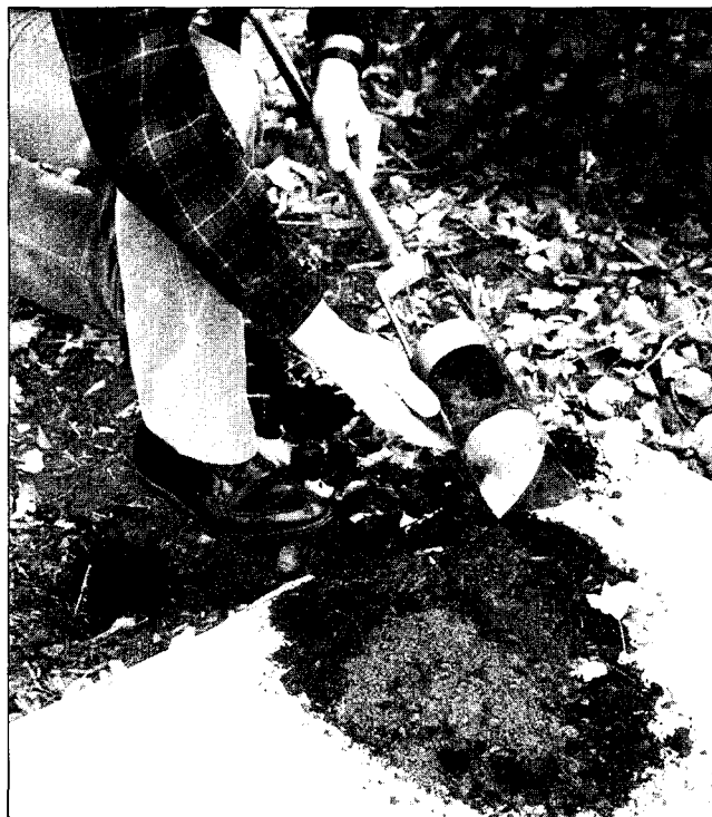
Figure 2. A hand-operated bucket auger collects a relatively undisturbed sample, allowing proper evaluation of soil texture and observation of possible mottling.
