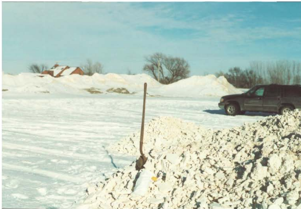
Figure 45. Mankato water treatment plant filter cake stockpiles.
