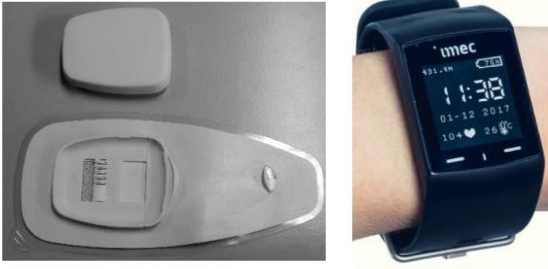
Fig. 3.10: Customized chest patch supporting two-lead ECG acquisition (left) and wristband with green LED PPG component.
