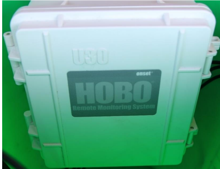
Figure 51. Data acquisition unit used to record soil moisture, rainfall and temperature during monitoring.
