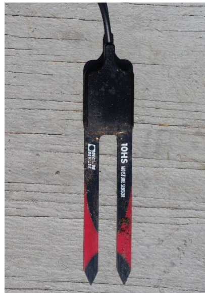
Figure 52. Typical soil moisture probe used for monitoring.
