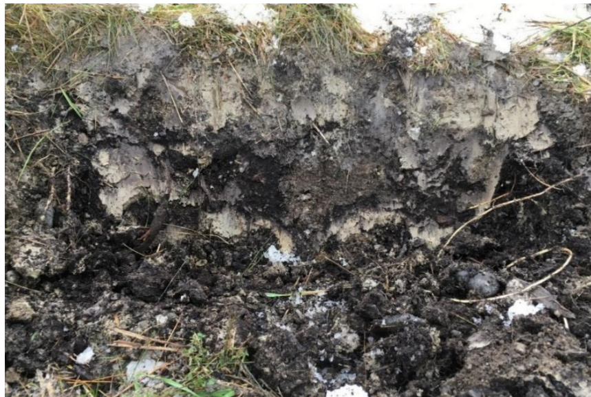
Figure 27. Characteristic soil profile from the Cook biofilter.
