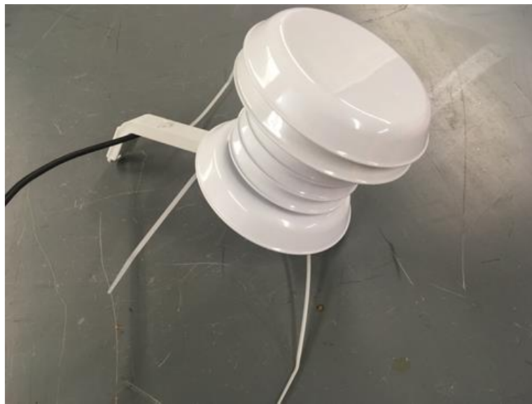
Figure 53. Rain gauge monitoring unit.
