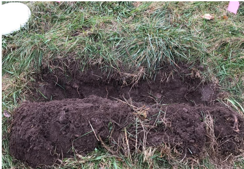
Figure 39. Characteristic soil profile from the Keene Creek biofilter.
