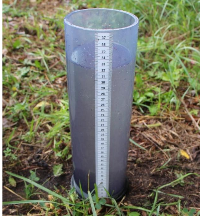
Figure 47. Modified Philip-Dunne Infiltrometer.
