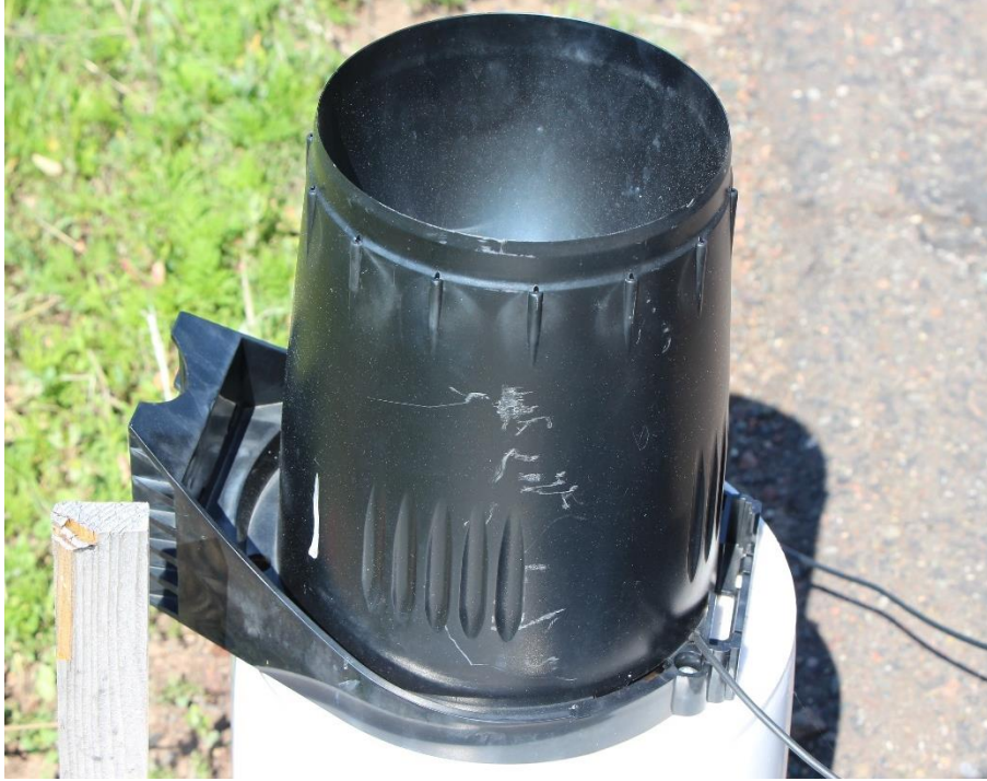
Figure 53. Rain gauge monitoring unit.
