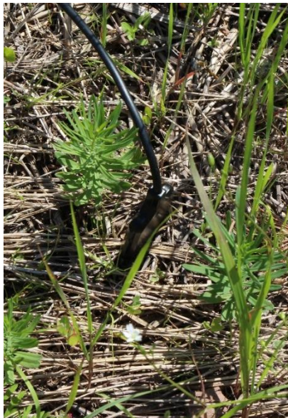
Figure 52. Typical soil moisture probe used for monitoring.
