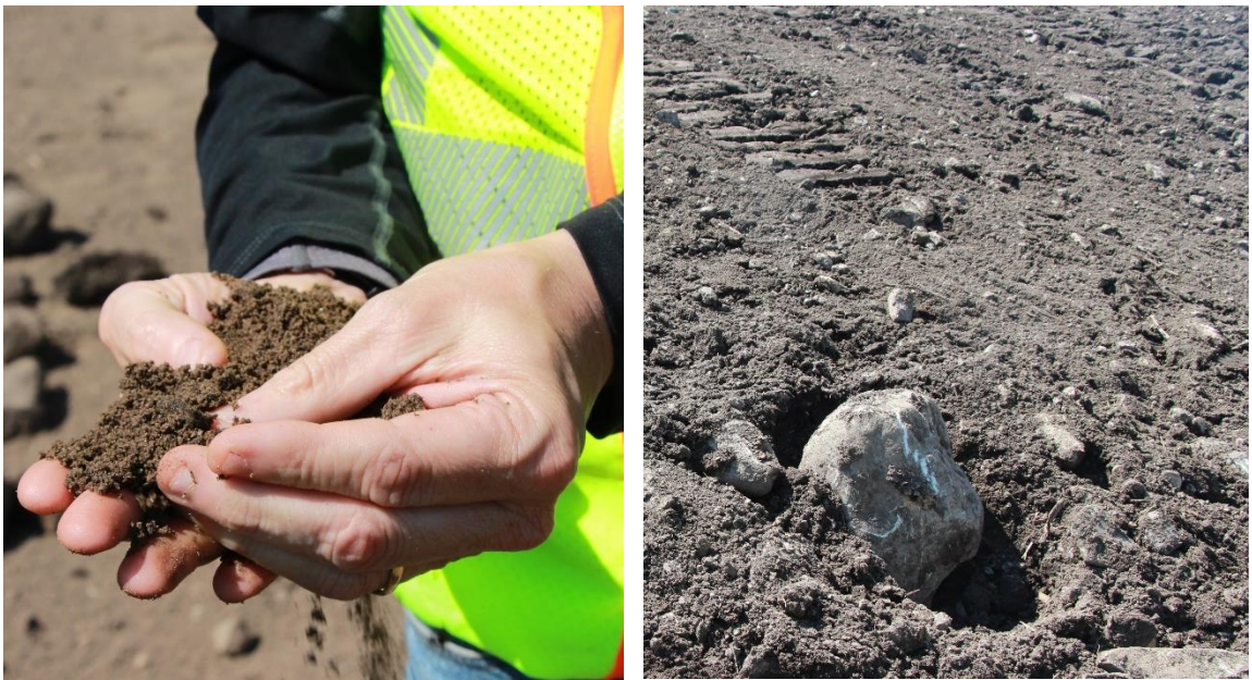
Figure 58. Typical sample of peat used at the Eagles Nest Project site.
