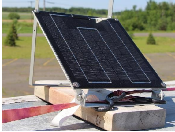
Figure 55. Solar panel used to sustain long term monitoring.
