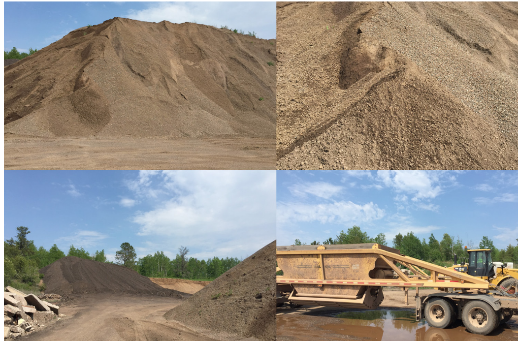
Mounds of RAP at a gravel pit in Carlton County offer road agencies an alternative to natural gravel and crushed aggregate for gravel roads. But RAP has to be used in the right proportion with gravel.
