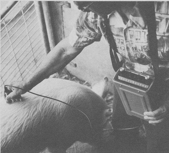
Figure 4b. Ultrasonically measuring for backfat thickness.
