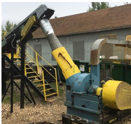
**Figure 3:** Oversized (+ 3/4 inch.) chips being fed to the chipper.
