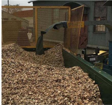
**Figure 4:** Oversized (+ ¾ inch.) chips collected after being resized by the chipper.
