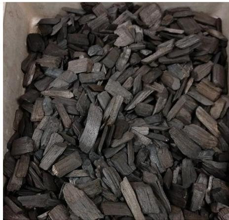
**Figure 5:** Picture of torrefied wood chips.
