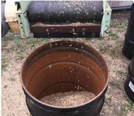
**Figure 2:** Undersized (-4 mesh.) chips collected after screening.
