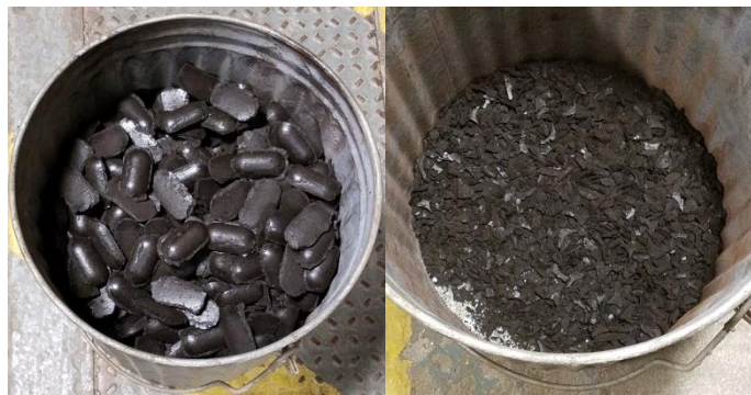
Figure 6. Pictorial of the briquettes retained on the screen and the fines passing.
