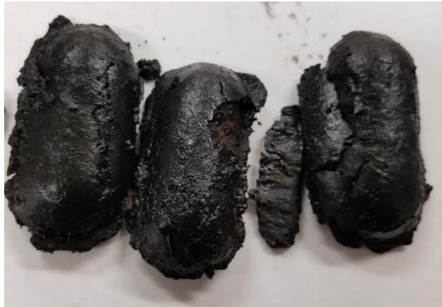
Figure 18. CS-6 sample; this briquette group displayed the least amount of moisture uptake, and before immersion had a more specular (shiny) surface.
