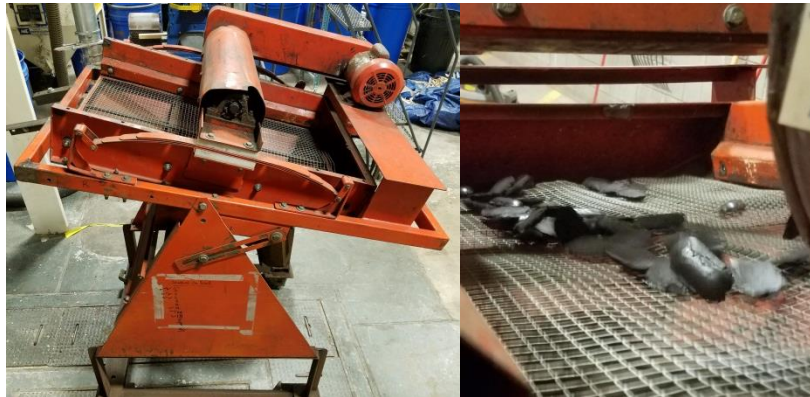
Figure 5. Vibratory screener and picture of briquettes during process.
