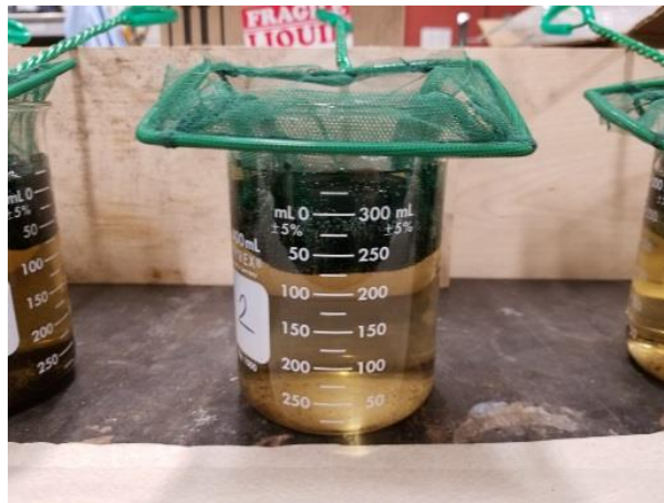
Figure 8. Visualization of water immersion and uptake procedure.
