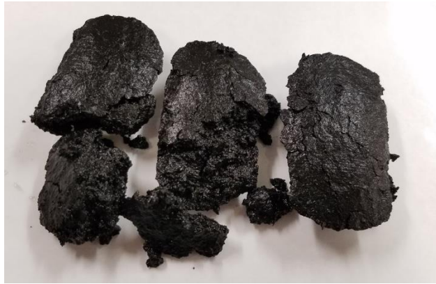
Figure 17. CS-8 sample; this picture best represents the state of most of the briquettes after they are removed from immersion in water after 24 hrs.
