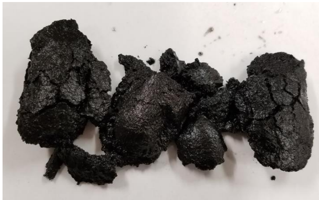
Figure 19. CS-10 sample; this picture best represents the level of disintegration that the samples CS-0, CS-7 and CS-10 displayed after 24 hours of water immersion.
