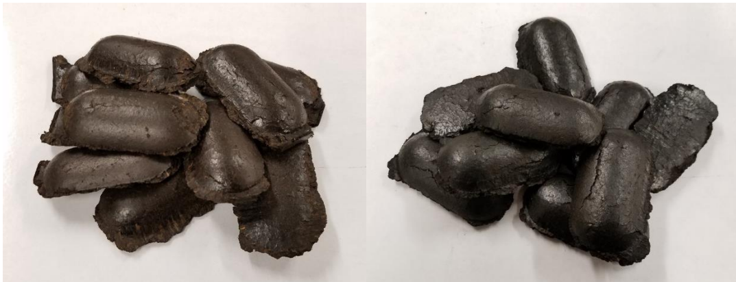
Figure 10. Visualization of the briquette product. CS-0 and CS-10 briquettes (left) consisted of t-wood that had a lower heating value and different particle distribution than the t-wood CS-1 through CS-9 (right) had.
