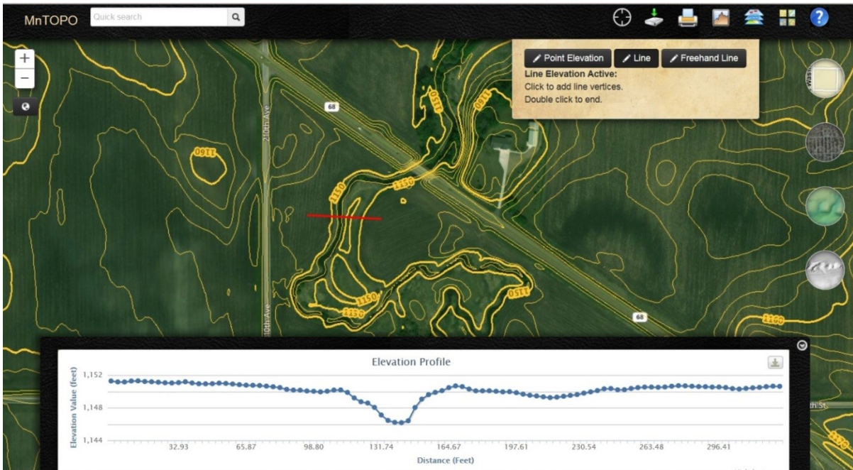
Figure 3.5.3. Example of MnTOPO LiDAR data. The elevation profile (stream cross-section along the red line) is helpful in showing the general shape of the stream and valley, however, a field survey is necessary to adequately capture the streambed.
