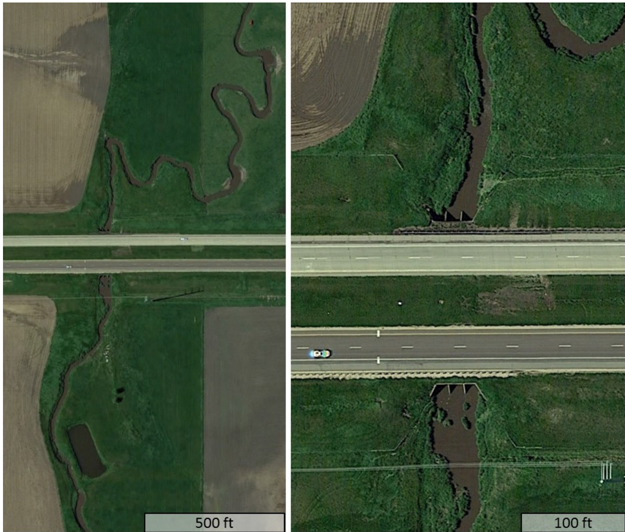
Figure 6.1.2. Highway I-90 over Elk Creek, near Magnolia, MN showing a triple barrel box culvert with inverts at the same elevation. The culvert is significantly wider than the upstream channel; the channel widens as it approaches the triple box culvert (flow from top to bottom). Vegetation-covered sediment is present upstream and downstream of the culvert indicating deposition. Google Maps images.
