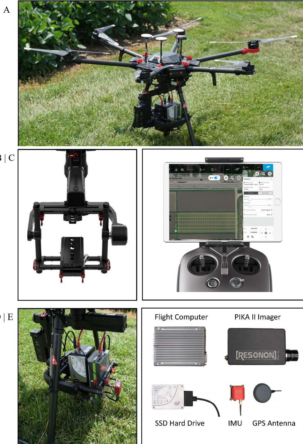
Figure 5.2. (A) Unmanned aerial vehicle: DJI Matrice 600 Pro equipped with A3 Pro flight controller. (B) Gimbal: DJI Ronin-MX. (C) DJI Ground Station Pro. (D) Airborne hyperspectral imaging system mounted on the gimbal. (E) Components of airborne hyperspectral imaging system.
