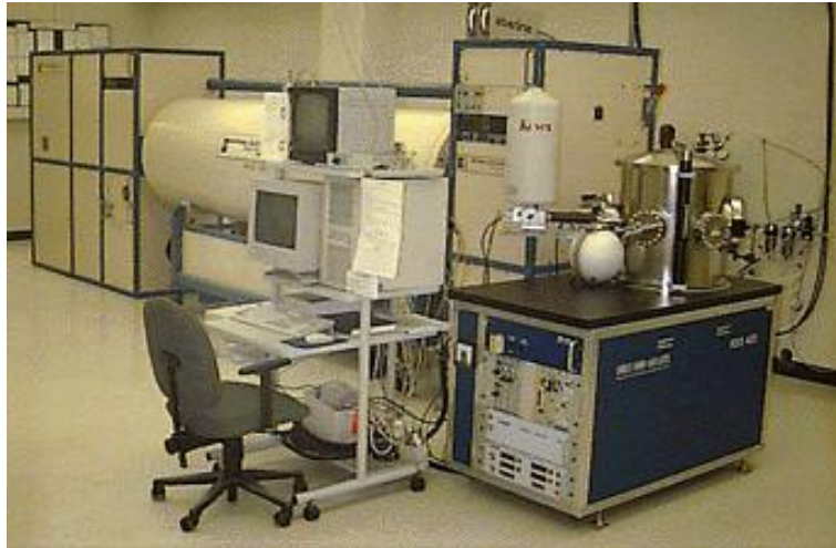
Figure 3.5: Ion beam facility with particle accelerator used for radiation testing (Source: University of Minnesota Characterization Facility).
