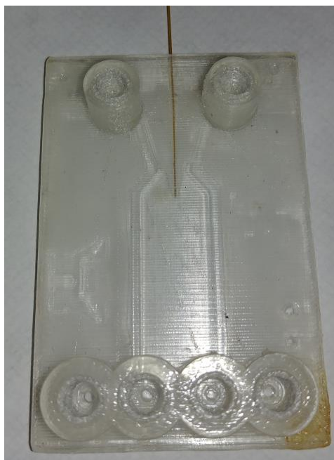
Figure 5.2 3D printed \mu FFE device in ABS plastic. The device is fabricated as a top and bottom piece. Both halves are then exposed to acetone vapor and pressed together to form a bond between the two pieces. Holes are drilled in the device and platinum wires inserted as the electrodes in the side channels. The capillary is sealed in place in the bonding step by placing it between the two layers. This particular device was printed and assembled in two days.
