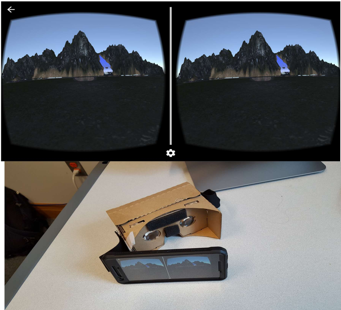
Figure 10: Mobile-based SMR-based BCI application. Bottom: Google Cardboard device for mobile-based VR applications
