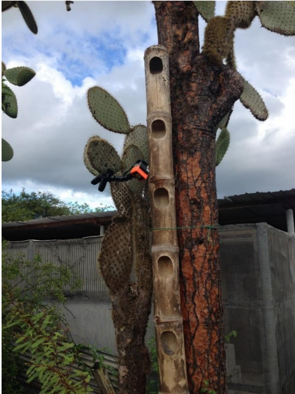
Figure 1.2. Set up of the video camera with an extended-life battery (orange), protective casing and flexible clamp mount facing the entrance of an active Galapagos flycatcher nest.
