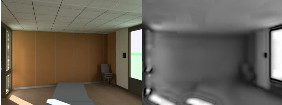
Figure 26. An example of intense image artifacting that occurs in the version of the prototype algorithm used in this experiment. The light band on the floor has strong contrast from rings that are introduced by image processing in the DEVA algorithm's simulation of Low Vision. More recent versions of the prototype have much less pronounced image artifacts, but participants did not view stimuli generated with those later versions.
