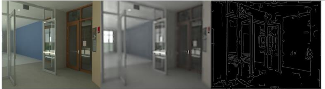
Figure 11: An illustrative example showing a scene, a severe Low Vision simulation, and the luminance boundary detection of that simulation image. The DEVA algorithm performs this step by using a Canny edge detector on the Low Vision simulation image.
