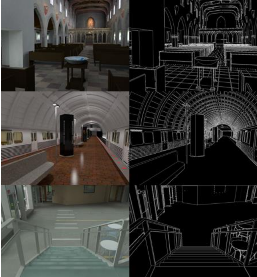
Figure 10: Examples of geometry boundary maps built from HDR scenes and CAD files. The prototype algorithm employs a robust process that detects geometry boundaries in a scene. The geometry-boundaries algorithm selects nearly every geometry boundary in a scene: far more than any one participant is likely to select.
