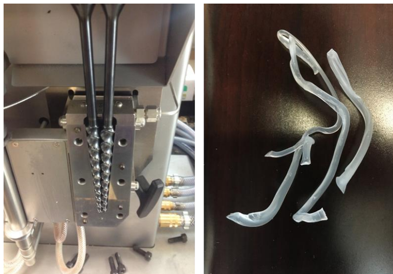
Figure 2.3 DSM Xplore microcompounder with circulating and conical twin-screws (left) and extruded samples after water cooling and drying (right).
