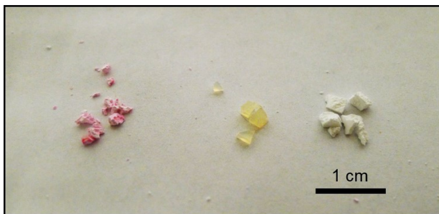
Figure 3.5. Photograph of a monolith prepared using 50 vol% 35\text{ kg mol}^{-1} PEO (left), a mesoporous P(S- co -DVB) monolith prepared without any PEO (middle), and a macroporous P(S- co -DVB) monolith prepared following a reported procedure using dodecanol as the porogen (right). 26 All monoliths were soaked in deionized \text{H}_2\text{O} with red dye for 24 h and then dried under reduced pressure.
