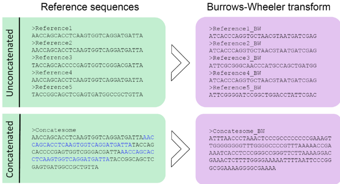
Figure 14. Burrows-Wheeler transform on concatenated sequences. Example of the Burrows-Wheeler transform on both small sequences (top) and a concatenated longer sequence (bottom). The concatenated sequence is more easily searchable using the LF walk. NINJA forms a BWT-compatible concatenosome that can be used interchangeably among various BWT-based aligners as an artificial reference chromosome. This concatenated sequence serves as a reference against which environmentally-obtained marker sequences are aligned.
