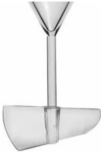
Figure 29. Rapid Visco Analyser paddle (www.perten.com)
