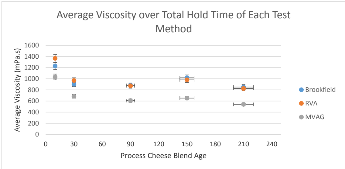
Figure 6. Average viscosity over total hold time (initial-4 hour) of each test method
