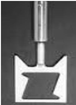
Figure 28. Brabender Micro Viscoamylograph spindle (Soon Suh and Jane, 2003)
