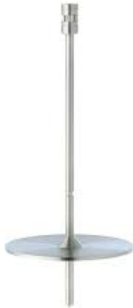
Figure 31. Brookfield rotational spindle ( www.coleparmer.com )
