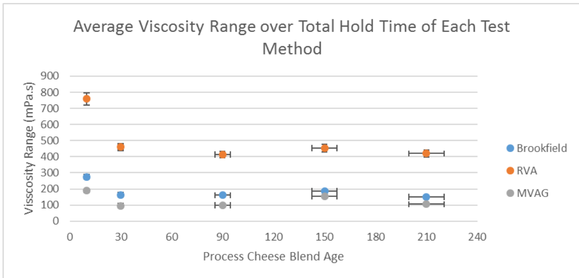
Figure 7. Average viscosity range (peak-low) over total hold time (initial-4 hour) of each test method
