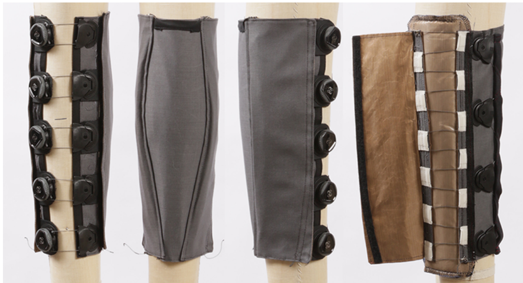
Figure 2.1: Shape memory alloy activated compression garment (SMA-CG) : For more information on garment design, refer to [5].
