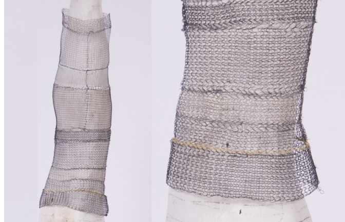
Figure 5.13: Active-Contracting, Variable-Stiffness SMA Knit Garment Prototype in an Unactuated State: (left) Front view, full garment. (right) Side view, thigh closeup. The prototype garment was knit according to the specifications in Appendix B.
