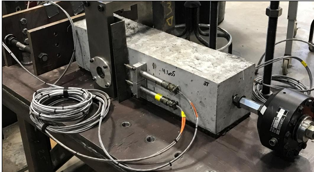
Figure 6-5. Direct tension test conducted as an extra step to this work.
