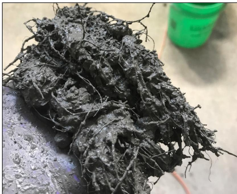
Figure 4-4. Fiber balling in a concrete mixture.
