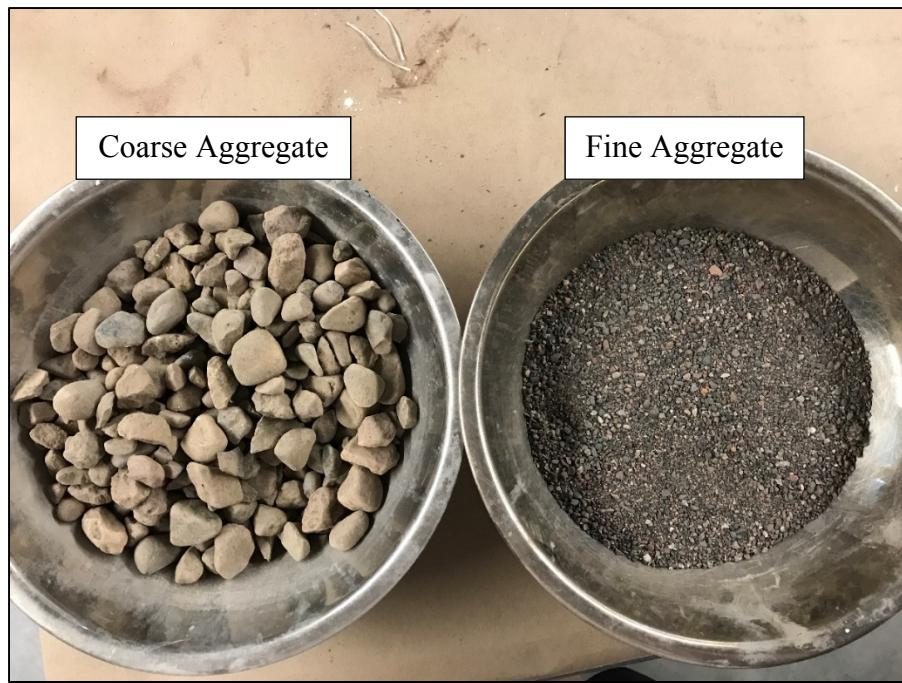
Figure 4-1. Coarse aggregate and fine aggregate used in this project.
