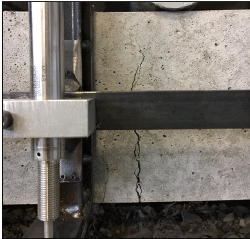
Figure 4-10. An example of a crack developed after peak load was achieved in a flexural performance test.
