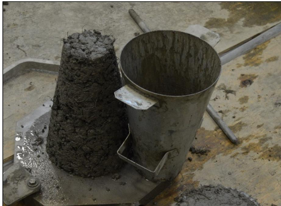
Figure 4-5. Slump test on FRC mixture.
