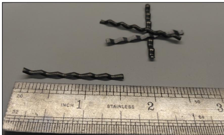
Figure 2-3. Steel fibers with crimped geometry in whole length.
