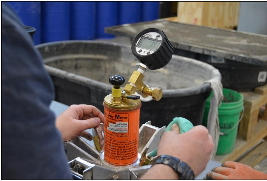
Figure 4-6. The air content by pressure method test is in progress.
