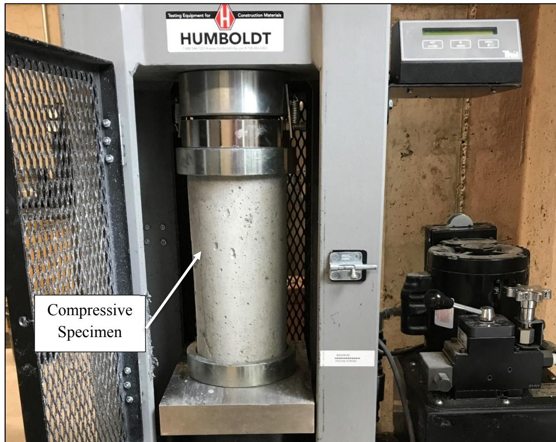
Figure 4-7. An example of a concrete compression test per ASTM C39.
