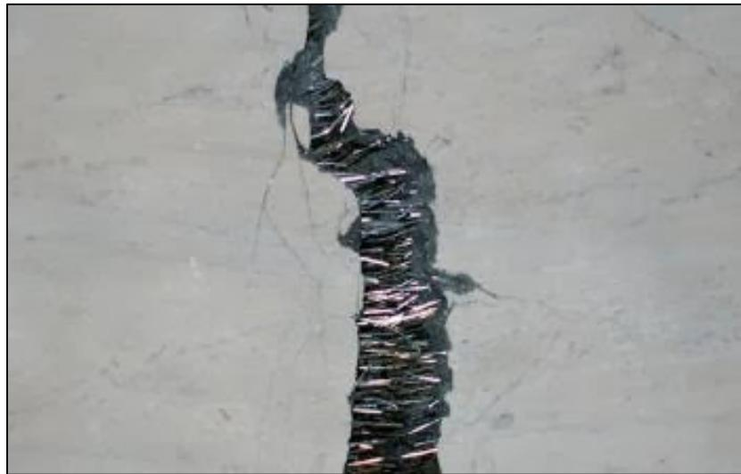
Figure 2-10. Fibers bridging a crack and providing post-crack performance (Gaddam, 2016).
