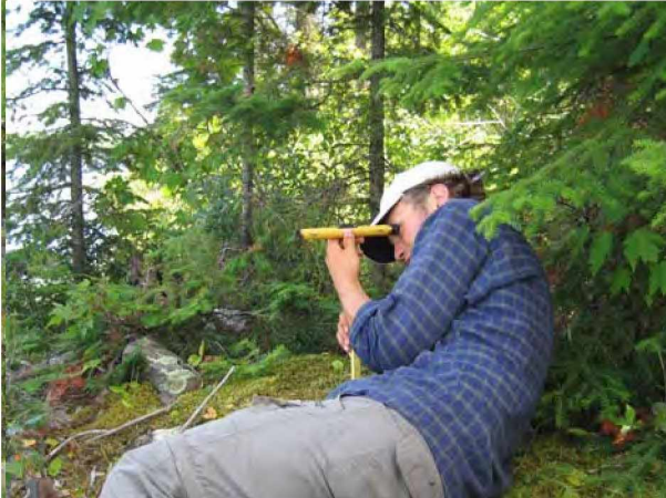
Viewing stadia rod through hand-held eye level
