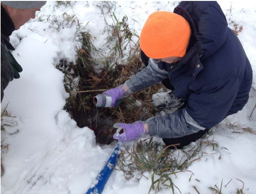
Figure 4. After priming the sinkhole with roughly 100 gallons of water, sulforhodamine B dye was introduced and back-flushed with additional water.
