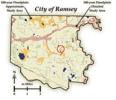
Map showing minor floodplain delineation changes impacting existing structures along a backwater to County Ditch #66.
