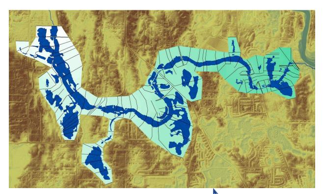
The modeling approach is illustrated here. The DEM raster landform elevation is the basis for the analysis (bottom layer). The modeled TIN is converted to a raster (middle layer). The raster analysis produces the floodplain result (top layer).
