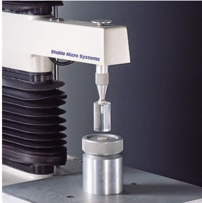
Figure 4. Chen Hoseney Stickiness rig used for measuring dough stickiness
