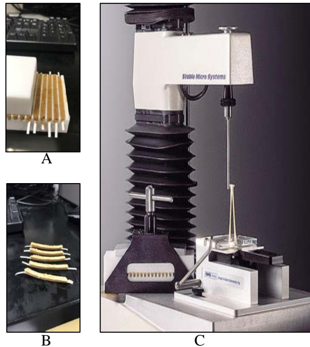
Figure 3. A. Dough strips formed as a result of compression of dough on the mold, B. Dough strips, C. Kieffer extensibility rig with the hook pulling the dough sample.
