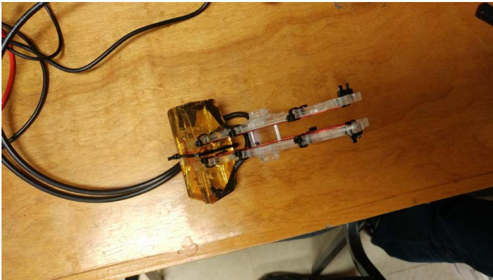
Figure 3: Photograph of actual prototype sensor. Main components of the sensor can be easily identified: the yellow transparent block contains connections between the legs of the sensor (orange wire on
