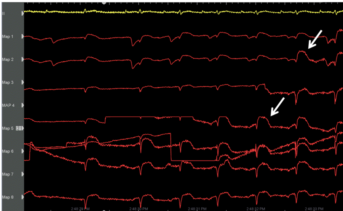
Figure 26. Shown here are representative waveforms from the prototyped catheter. These channels are representative of the unipolar MAP recordings. The white arrows indicate representative monophasic action potential waveforms. Amplitudes for these waveforms range between 1-3mV.
