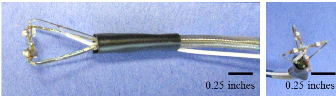
Figure 29. The electrodes array from a multi-array ablation catheter was modified such that there were only 4 electrodes instead of 8 to increase contact force.
