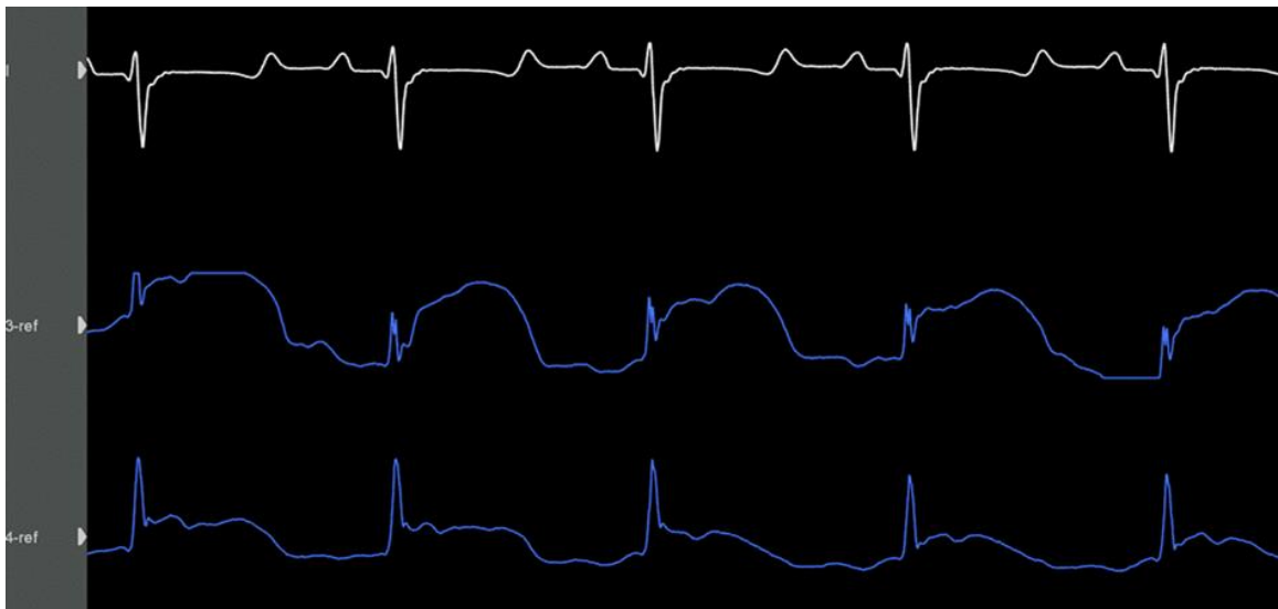
Figure 38. A second generation pericardial mapping prototype was used on the right ventricular epicardium of an in situ swine heart. Waveforms representative of monophasic action potentials were recorded on bipolar pairs between electrodes 3 and 4 and a non-contact reference electrode.
