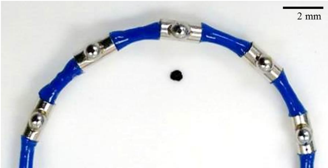
Figure 24. A pulmonary vein ablation catheter electrode ring was modified through the addition of small balls of conductive material to the existing base electrodes.
