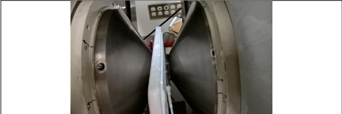
Figure 3.5b the microstrip test circuit inside the Electromagnet with spacers to hold it in place.
