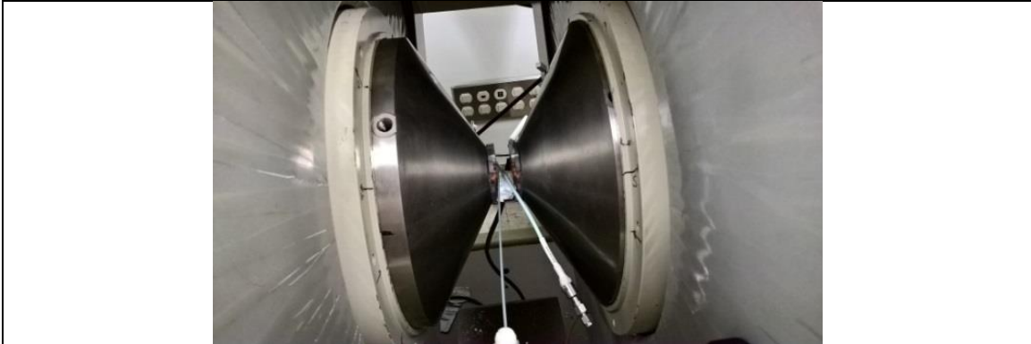
Figure 3.4b the Electromagnet core with VNA cable
