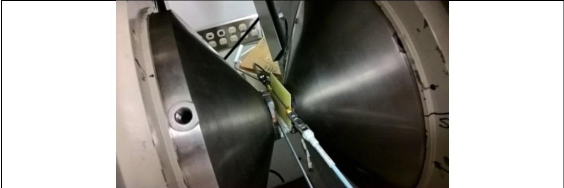
Figure 3.5a a microstrip test circuit inside the Electromagnet
