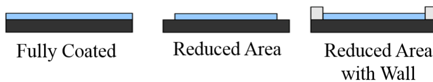
Figure 3.11: Schematic diagram for the cross section view of coating samples run using finite element method.
