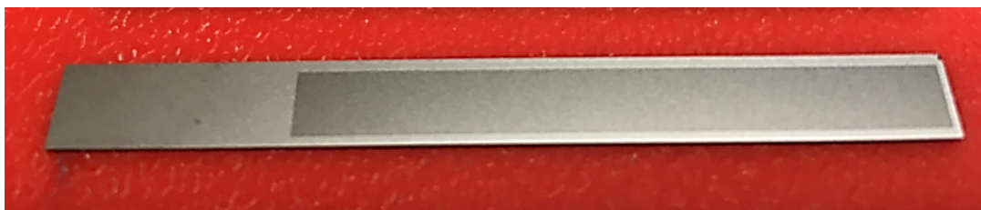
Figure 7.2: Photograph of the cantilever using for beam deflection stress measurement. The cantilever is made from standard silicon substrate (dimension of 6 mm \times 60 mm with thickness of 520 \mu\text{m} ) with a coating area (5 mm \times 45 mm) etched-in 17 \mu\text{m} in depth.
