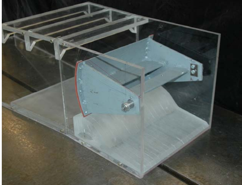
Figure 2.11. The original geometry of the existing spillway and the tainter gate which were made of acrylics and sheet metal, respectively.
