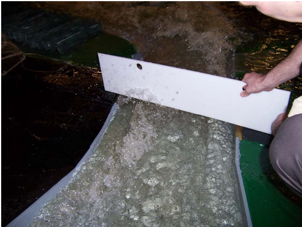
Figure 3.20. Under the spillway Design-2, but with no bridge in, water flowed through the channel without overtopping the side walls. By placing a plastic board over the channel walls the standing wave hit the board and splashed over the west side wall
