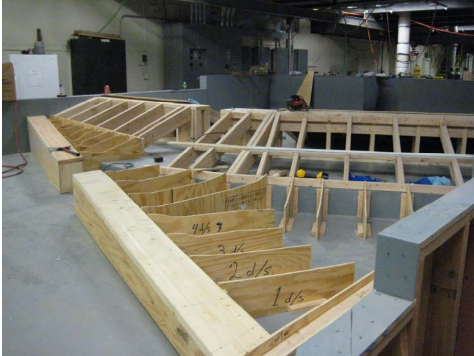
Figure 2.9. The physical model of the Bond Falls spillway system under construction. The embankment, road, topographic templates and structural elements were built from lumber and plywood.
