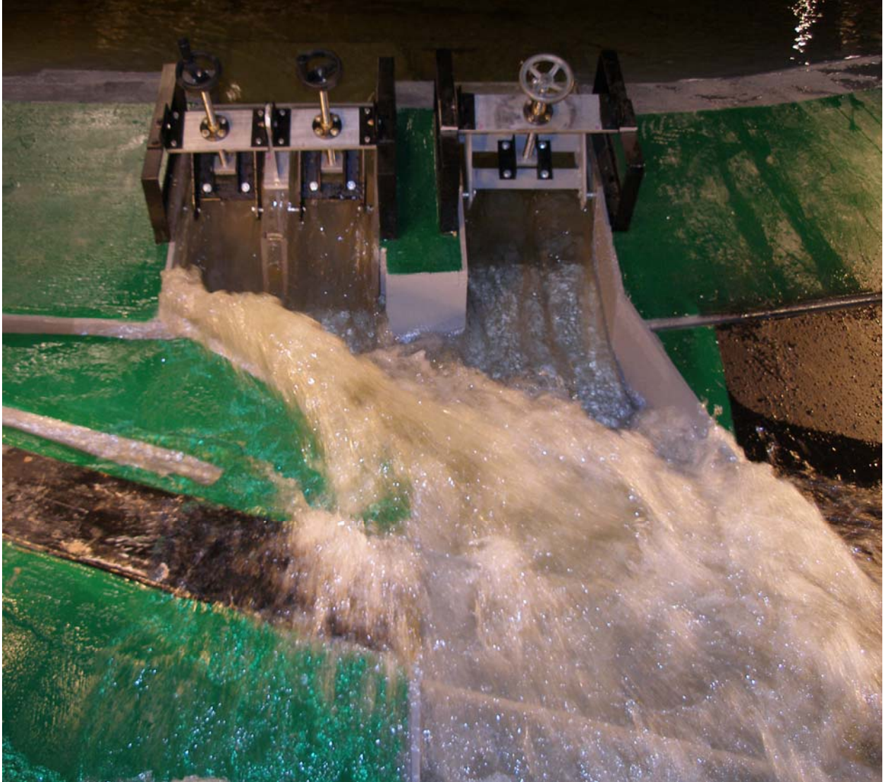
Figure 3.9. Water flowing through the spillway Design-1 under the PMF (flow). All three gates are fully open and the reservoir is at the maximum pool level (1480.9'). Under this condition, flow overtopped the 50° wall downstream of the new gates (on the left side of the picture) by 16 ft and the west side wall upstream of the bridge (on the right side of the picture) by 8 ft.
