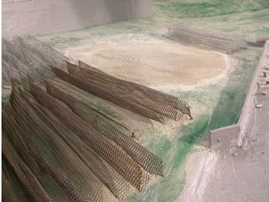
Figure 3.5. The elevation of the area behind the retaining wall was increased to more accurately reflect the topography of that area. In addition, chicken wire was added to the channel floodplain to model the roughness of the wooded areas in the prototype.
