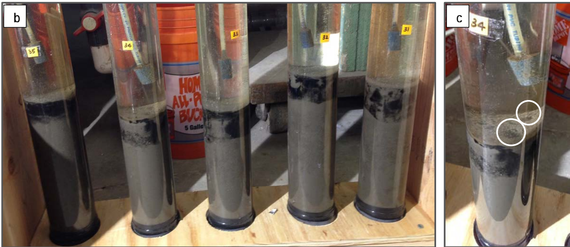
Figure 23. Ann Lake column studies on high sulfate in the water column. (a) Mean water column sulfate concentrations ( \pm 67\% CI) in the control and iron-amended sediment columns. (b) Photograph of control columns containing high sulfate in the water. (c) Photograph depicting craters on the surface of the sediment due to gas ebullition.
