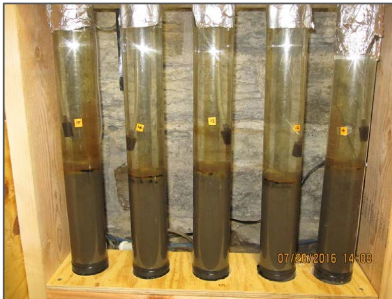
Figure 19. Ann Lake sediments amended with 0.1 g/cm 2 iron filings under oxic water column conditions. The oxidized iron layer can be seen at the sediment-water interface.
