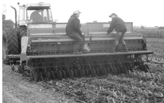
Photo 1. No-till drill planting fall cereal rye.
