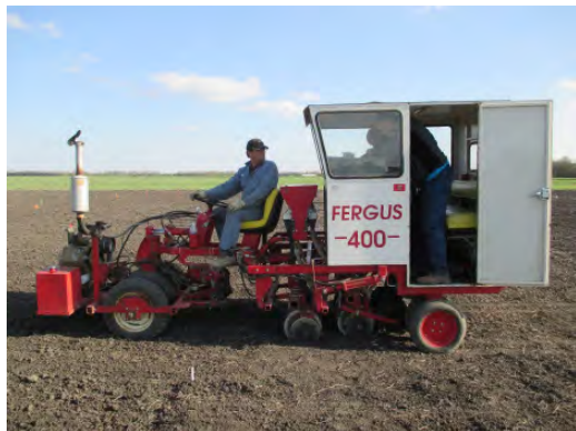
Figure 1. Mid-row banding of fertilizer materials with the help of Borgault unit for spring wheat during 2014 growing season at Glyndon, MN.
