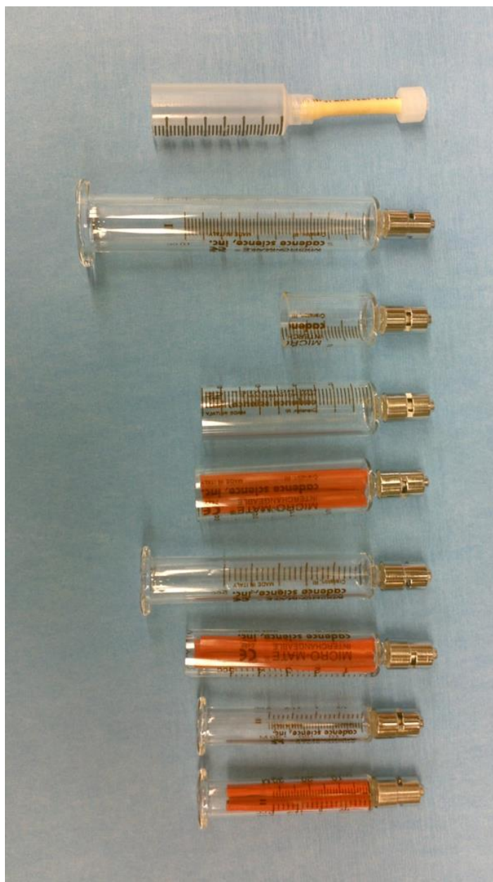
Figure F.6.1: Prototype outflow tubes v1. Picture of various prototype outflow tubes used to prevent the removal of cell-aggregates during perfusion culture in stirred suspension bioreactors. Syringes of various materials and diameters were tested with different “baffle” designs to prevent turbulence in the medium of the outflow tube. All of the tube designs were intended to maintain a volume of medium within the tube that is slowly removed with the linear vertical flow being slower than the settling rate of spheroids in culture. Turbulence was observed with all of these outflow tube designs that prevented proper function and did not prevent removal of aggregates in the perfusion waste stream.
