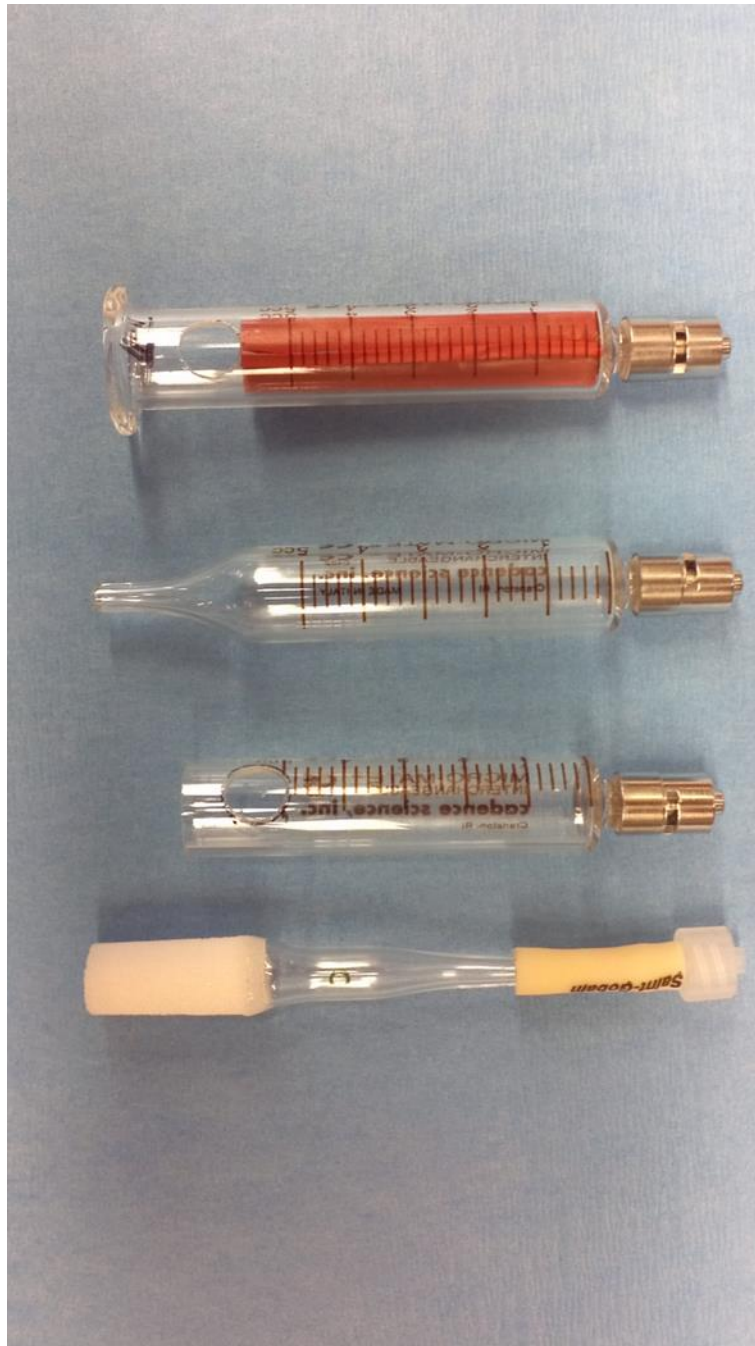
Figure F.6.2: Prototype outflow tubes v2. Second series of outflow tube designs tested with cell aggregate cultures in perfusion stirred suspension bioreactors. These designs incorporated more complex geometries to reduce turbulence that was observed within the first series of outflow tubes tested. The most successful tube was a porous “fritted” glass tube that maximized the surface area for medium removal which minimized clogging of the filter. The linear flow velocity through each pore in the filter was much lower than the settling rate which prevented clogging at normal cell/aggregate densities in culture. Some clogging was observed at very-high cell densities ( \gg 3.0 \times 10^9 cells/ml), and studies were designed to avoid this upper limit.
