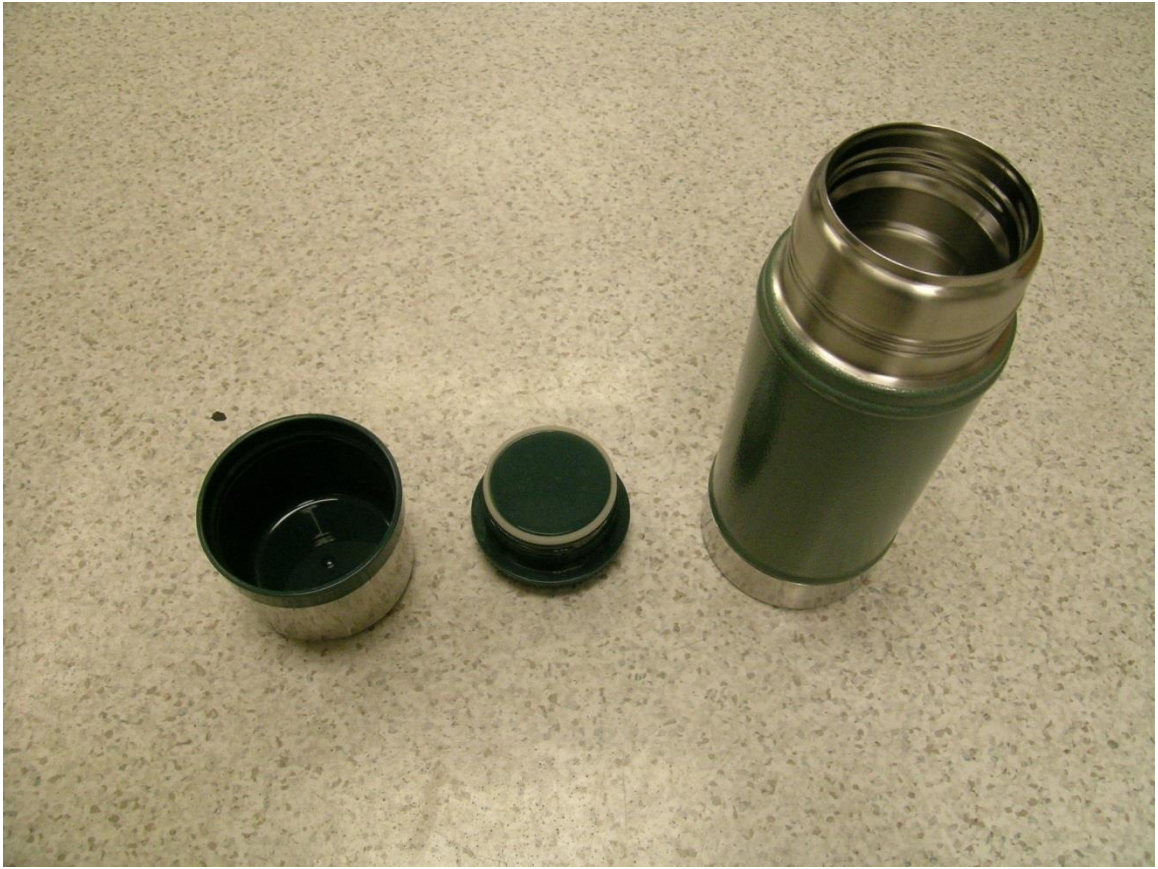
Figure F.D.5: Beverage container for temperature and pressure regulation. A thermos beverage container was proposed for maintaining temperature and pressure of islets during shipment, but was abandoned due to difficulty with form-factor.
