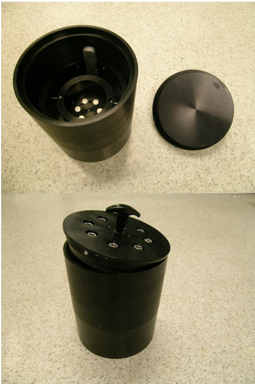
Figure F.D.6: Pressure regulated gyrosopic shipping container (PRGSC). A custom-built pressure regulated gyrosopic shipping container was designed and manufactured by Wilson-Wolf Manufacturing for studies to investigate the pressure effects on islets during culture and shipment. This container was designed to work with silicon rubber membrane flasks that function when they are properly oriented (upright), so a gyrosopic mechanism was included in the container to ensure ideal flask orientation during shipment. These devices were tested in a vacuum chamber to simulate the pressure changes experienced during shipment in the cargo-hold of cargo air-shipments.
