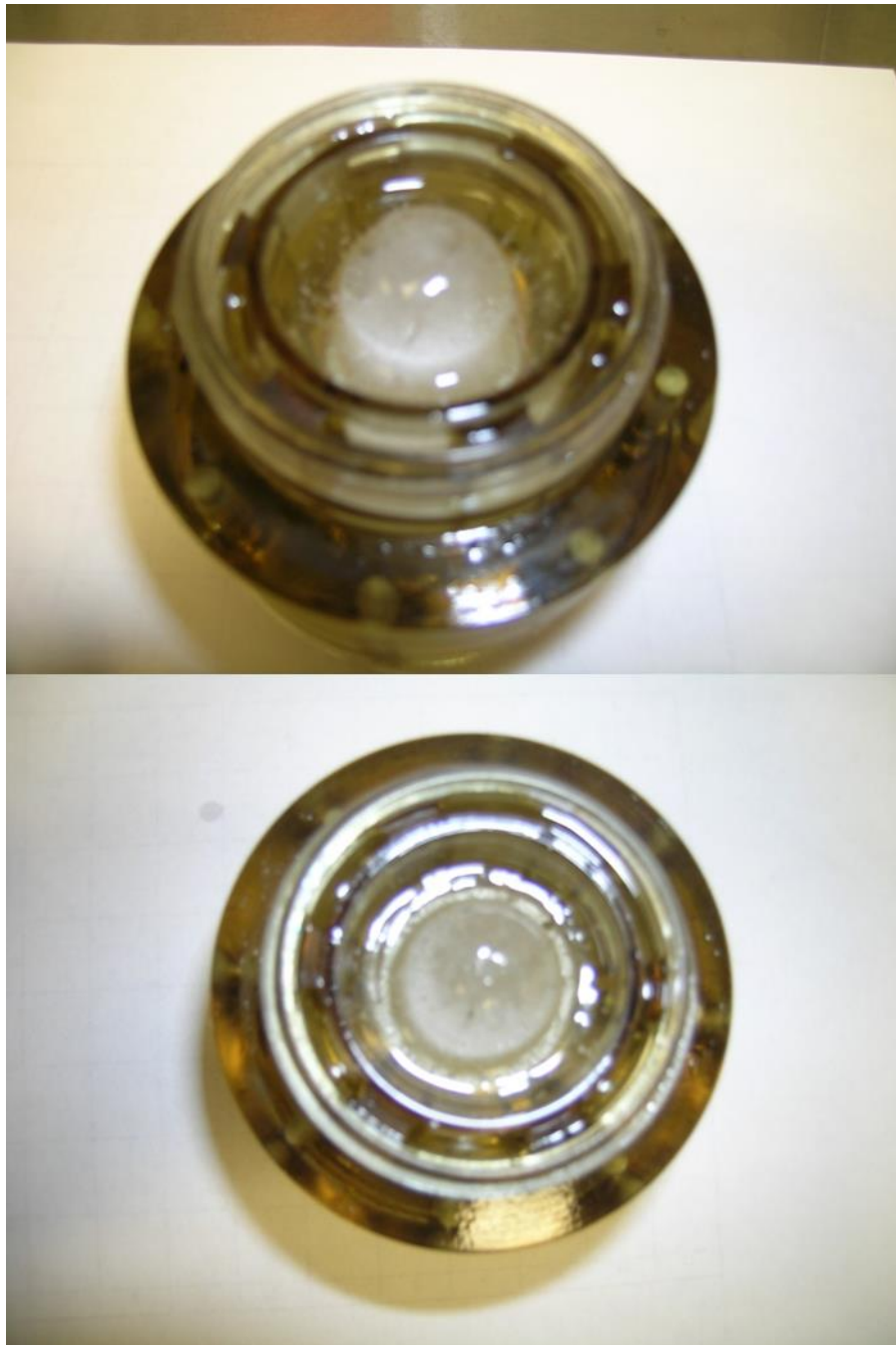
Figure F.D.1: First generation Wilson Wolf SRM culture devices. These images illustrate the importance of temperature regulation during islet shipment, and confirm that the culture vessel contents freeze solid when external temperatures are below -20\text{ }^{\circ}\text{C} for 24 hours.
