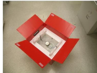
Figure F.D.3: Preparation of ThermaSure and TCP materials. The recommended preparation and loading of temperature stabilizing materials for islet shipment.
