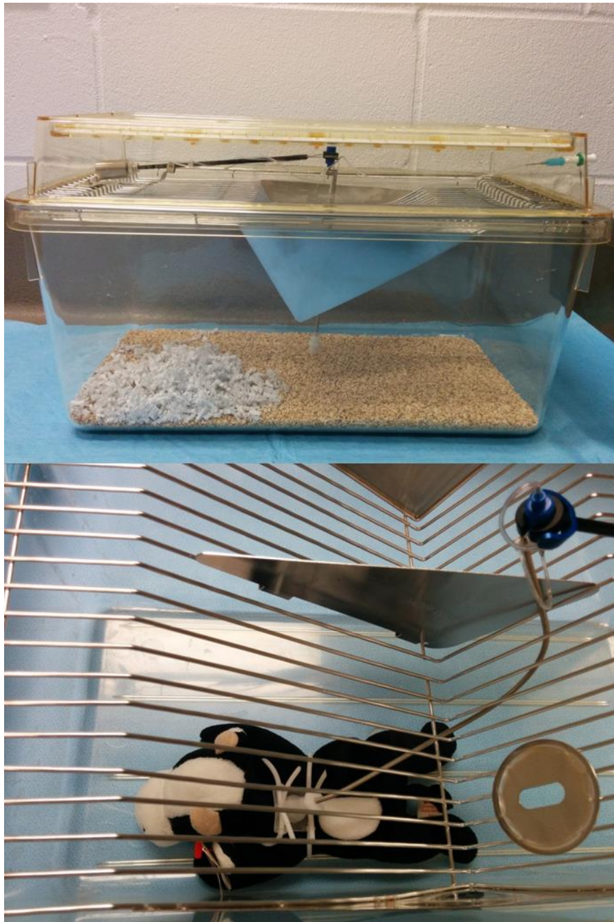
Figure F.8.8: Pictures of DSO harness and tether apparatus. A port was added to each cage lid for animals receiving DSO. The exterior port of the cage lid was connected to the DSO manifold, and the interior port of the cage lid was attached to the tether apparatus (Instech Labs.) The entire cage set-up with counter-balance, tether, and harness apparatus is picture on top, and view from above shows the tether apparatus attached to the dual-channel harness on the animal (animal is illustrated as a toy cow in photo).
