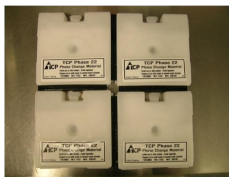
Figure F.D.2: ThermaSure and TCP temperature stabilizing materials. These two materials were tested for regulating temperature during islet shipment. The ThermaSure (TS) temperature stabilizing material was intended for maintaining temperatures between 16-20 °C and was originally intended for transporting blood products. The TCP Phase Change Material (PCM) was intended for maintaining temperatures between 20-22 °C, and was investigated as an alternative to TS material due to its improved thermal regulatory capacity and because the targeted temperature range coincided well with the standard culture temperature used for human islet cultures (22 °C).
