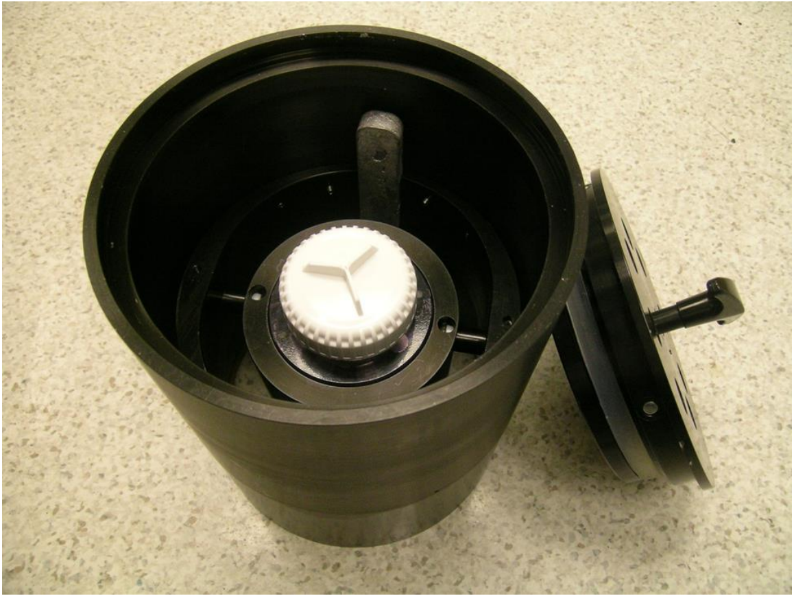
Figure F.D.7: PRGSC shown with SRM flask. The flask was held in position within the gyroscope using a strap and magnetic contacts. The lid created an air-tight seal with the cylinder to maintain normal atmospheric pressures (~760 mmHg) during shipment.
