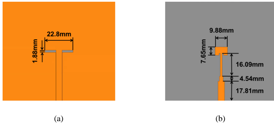
Fig. 3.14. Structure of two source antennas: (a) slot antenna (b) patch antenna
