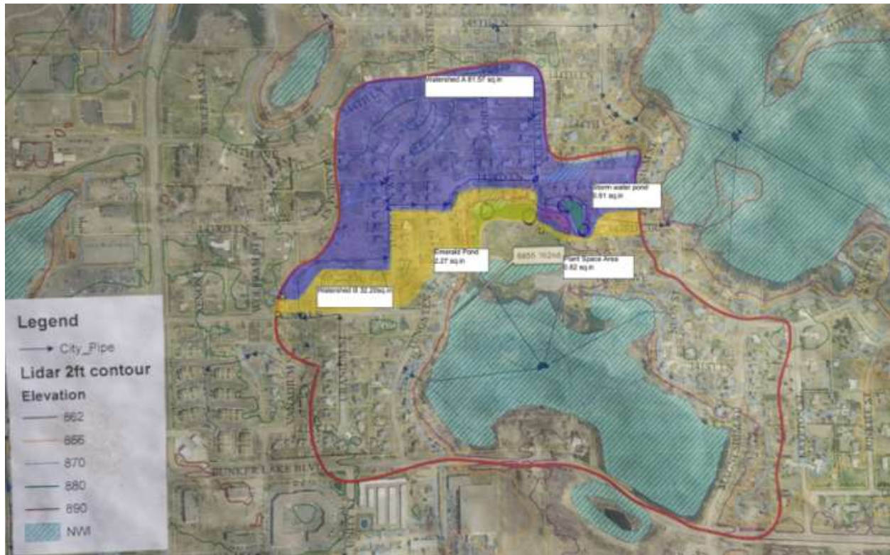
Figure 2. Subwatershed delineation. Watershed A in blue empties into Stormwater Pond. Watershed B in yellow empties into Emerald Pond.
