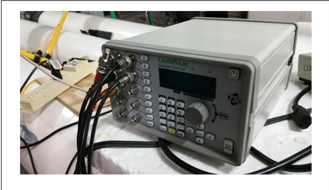
Figure 2-27: Picture of TSI model 610036 synchronizer box
