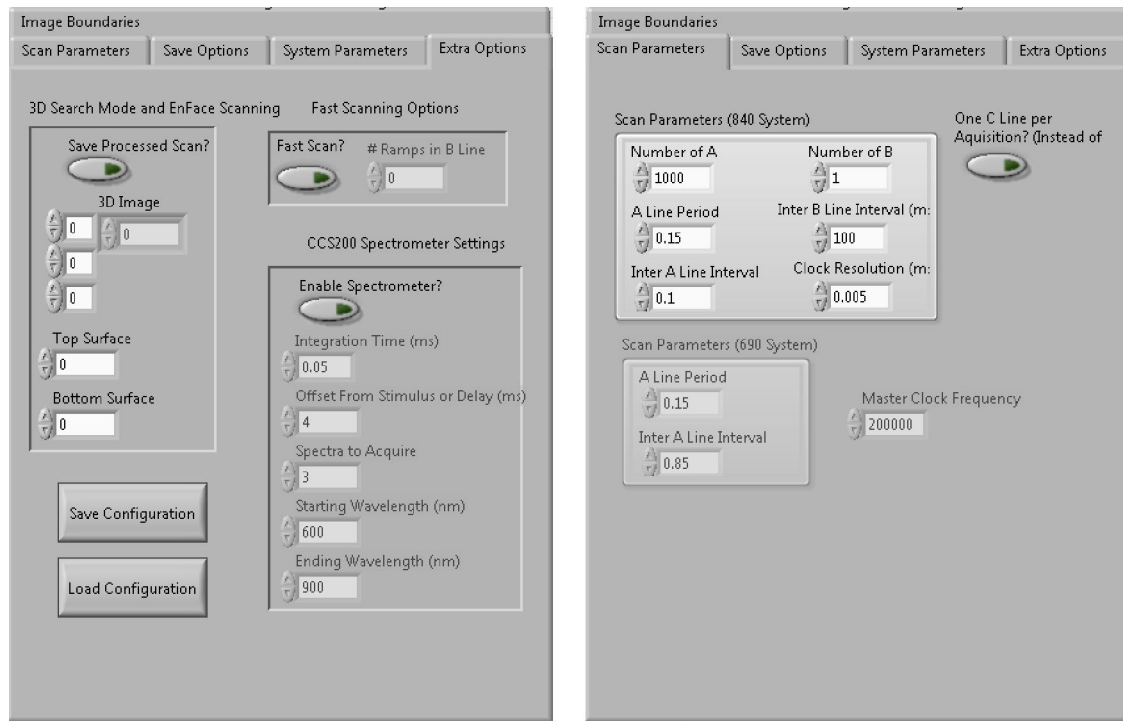
Figure 3.5. The front panel of the acquisition program demonstrating some of the options and parameters that can be used to customize acquisition.
