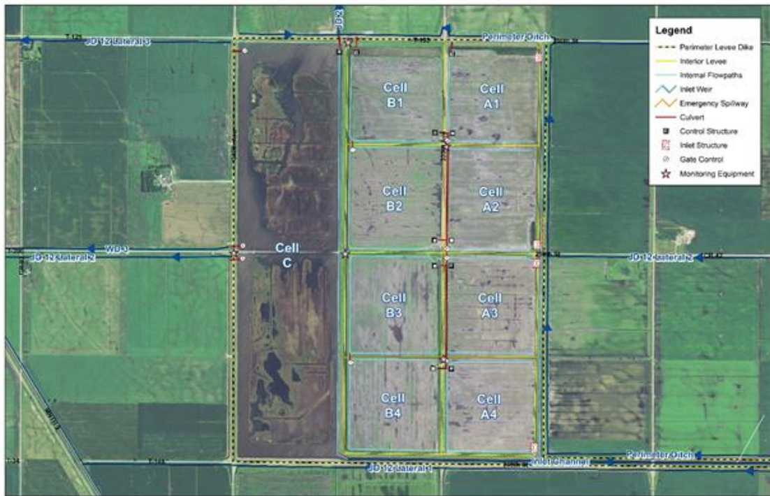
Figure 3. Interior diking plan for impoundment cells, showing cell names and structures (Ostlund 2016).
