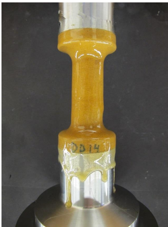
Figure 22. Polyurethane coated specimen with extension platens.
