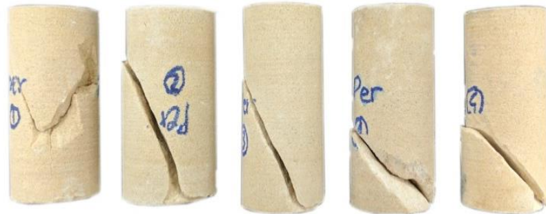
Figure 15. Shear failure of triaxial compression specimens at radial stresses of 2.5 (left), 5, 10, 20 and 30 (right) MPa.
