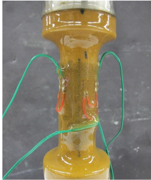
Figure 24. Axial resistive strain gages on dog-bone specimen.
