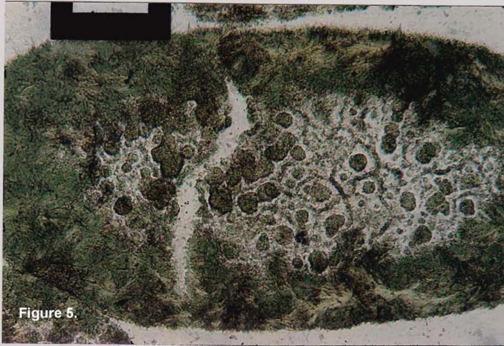
Plane light, Mag. 170X Outer granule is stilpnomelane, inner is greenalite grains and chert
