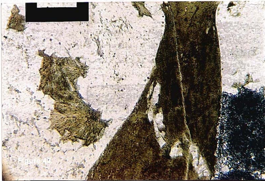
Plane light, Mag. 170X Stilpnomelane granule and radiating crystals, Carbonate, Magnetite in Quartz
