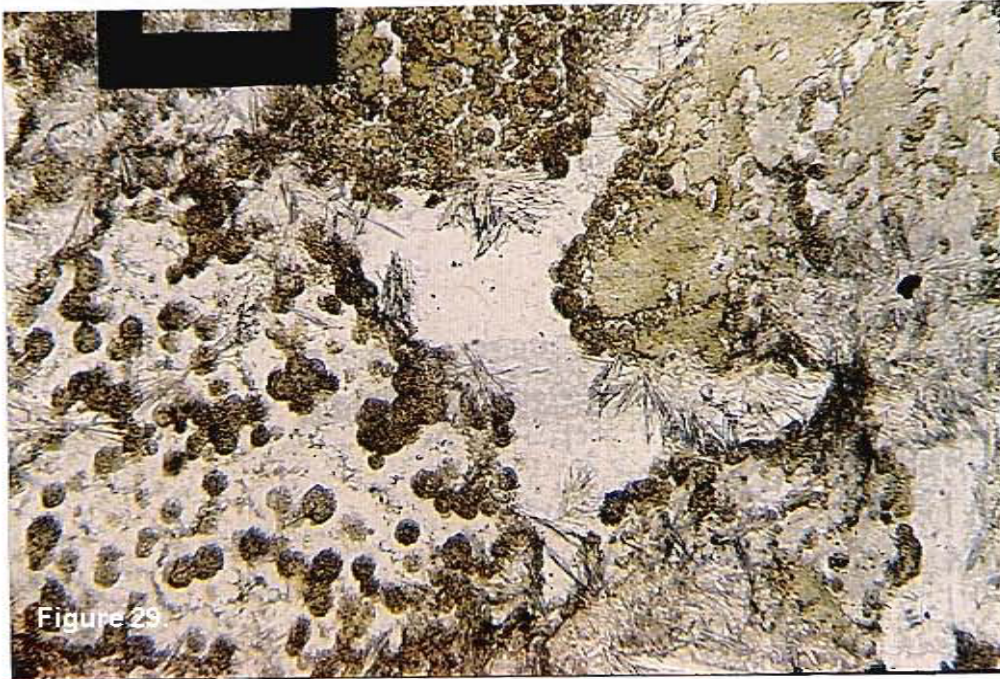
Plane light, Mag. 170X Acicular Minnesotaite-Quartz-Greenalite(fabric and grains)granules
