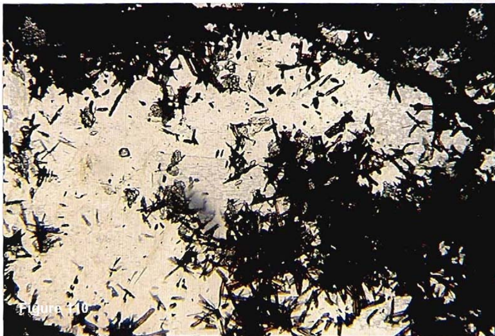
Figure 110 Plane light, Mag.170X Acicular Goethite and Magnetite in Quartz. Goethite is apparently an alteration product of Minnesotaite
